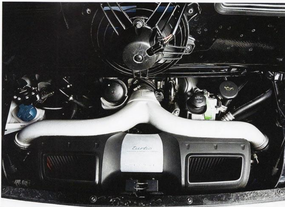
The modified 3.6-litre twin turbocharged flat-six produces 700 horsepower, giving the EVT-700 startling performance
