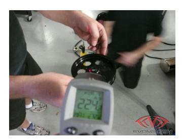
**Step 6:** Heat the EVOMS pulley in an oven, with a hot plate or propane torch. The exact temperature is not critical, however more heat will allow the aluminum to expand and install over the snout of the crank easier. **Wear hand protection to prevent getting burned.** Once hot, install onto the crankshaft – make sure to align the dowel pin on the pulley into the hole on the crankshaft
