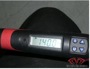
**Step 11:** Using a 19mm deep socket and calibrated torque wrench, tighten the pulley bolt while securing the pulley installation tool with a 36mm wrench. You will want to tighten the pulley bolt to 140 ft./lbs. of torque.
