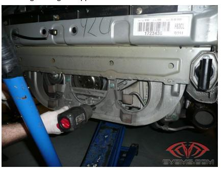
**Step 5:** Once the bolts are removed, remove the muffler support bracket and crank pulley
