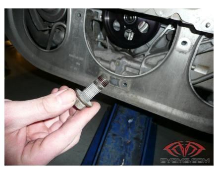
**Step 10:** Use the supplied EVOMS Billet Pulley Installation Tool (d) to secure the pulley while performing the final torque to the crank bolt. Align the dowel pins on the pulley installation tool into the holes on the pulley.
