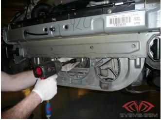
**Step 2:** Remove OEM crankshaft pulley. This can be accomplished by using the OEM crank pulley removal tool or with an impact gun. The crank bolt has a 22mm head.
