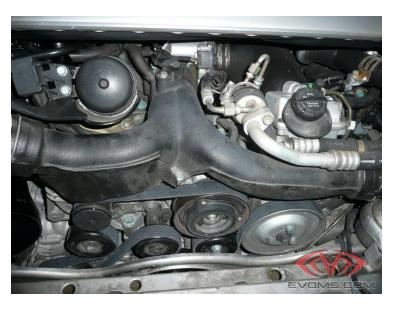
**Step 13:** Install the supplied Serpentine belt (turbo applications) or reinstall the OEM belt (GT3 applications). Be sure to route the belt in the same way as it was stock. See photos below.
