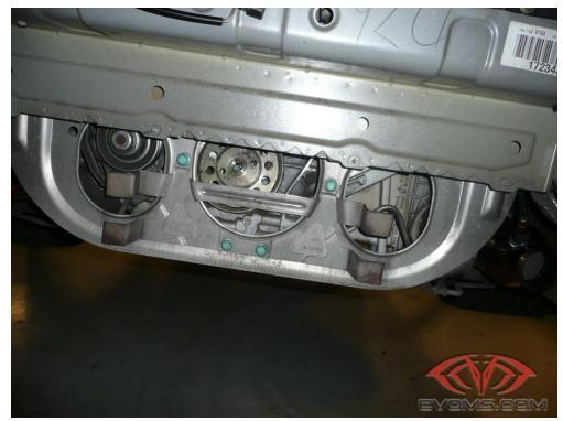
**Step 4:** Support the engine with a hydraulic jack before removing the engine support bolts.
