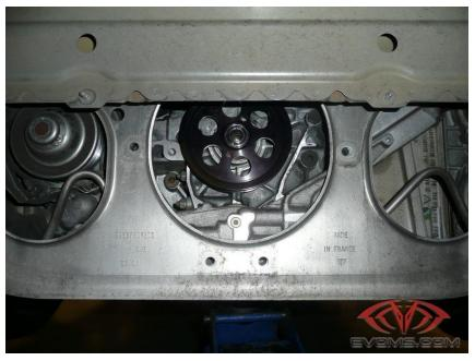
**Step 7:** Use the supplied Pulley Installation "Set Bolt" w/ Washer (e) to draw the pulley onto the crankshaft. The exact TQ specification for this step is not critical but the bolt should be snug.
