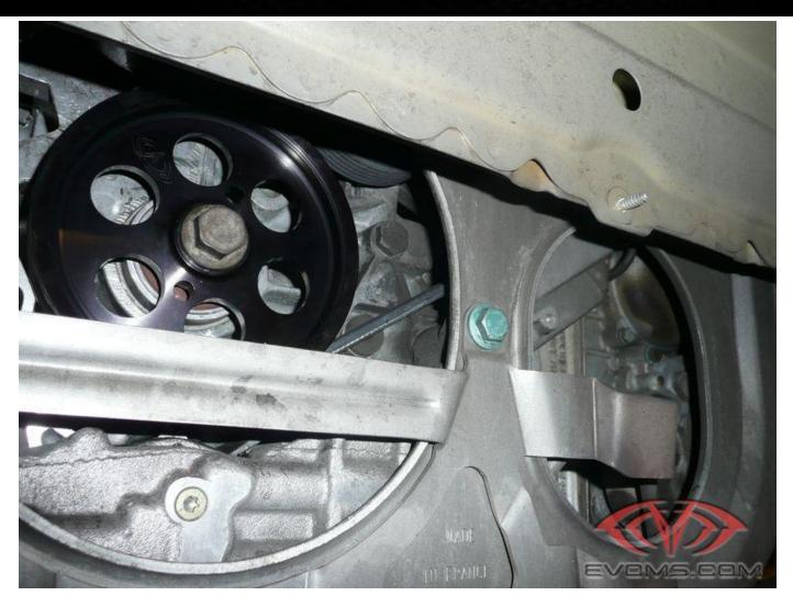
**Step 14:** Reinstall the exhaust and airbox. Start the vehicle and check to see that the belt rides properly on all of the pulleys. Once verified, reinstall the rear bumper.
