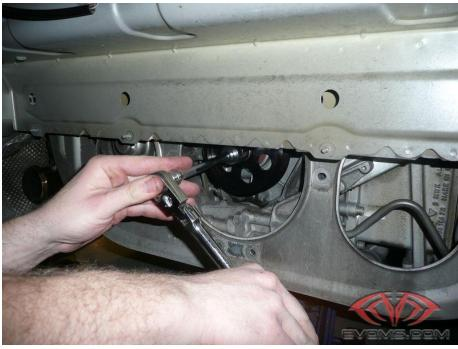
**Step 8:** Once the Pulley Installation "Set Bolt" w/ Washer (e) is tight, remove this bolt. This bolt is not used for the final installation and is no longer used.
