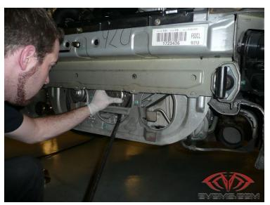
**Step 3:** Remove the OEM pulley. This may require using a pry bar to work the pulley loose. Once loose and off the snout of the crankshaft, it is ready to be removed. This will require removing the engine support / muffler support bracket. REMOVING THESE BOLTS REQUIRES SUPPORTING THE ENGINE WITH A HYDRAULIC JACK.
